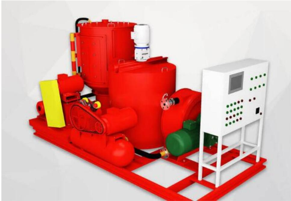
The GBP series of Automatic Bentonite Turbo Mixer/Pump Plant consists of a steel sheet cylindrical tank, set-up on a strong base frame, the pump and the motor. The muds are mixed through a high speed vortex produced by a special pump which, after sucking the material from the bottom of the tank, sends it back tangentially into the same tank in order to get highest possible efficiency.
