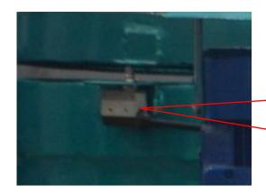
Travel switch, installed under the vibration, when remove the vibrating screen, equipment stop work; When maintenance and repair, it can prevent wrong operation.
