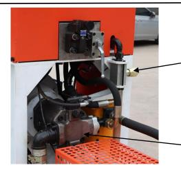
Adjustable output with this valve (LS control)
