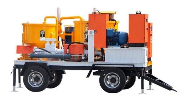
LGP400/1000/95/165DPL-E/A Grout mixer and pump with wheels are integrated with a screw feeder, mixing, agitator and horizontal hydraulic pump. It is mainly used to be made such as cement slurry or bentonite slurry, etc., for injecting in the sub-soil for soil consolidation, piling or even for long transport of material.
