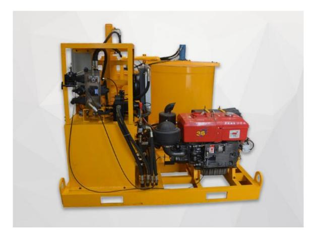
The LGP400/700/100PL-D grout station is combination of mixer, agitator and hydraulic plunger grout pump in one plant. Mainly suitable for mixing and pumping water, cement, sand, bentonite, filler, clay power, silicates and other additives.
