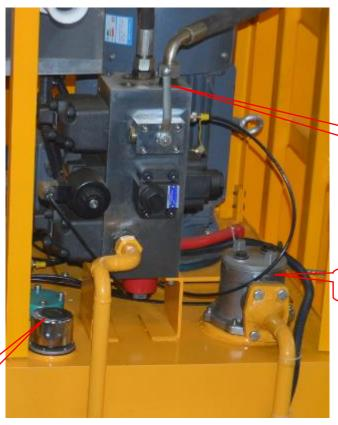
High speed and lower speed switch valve
