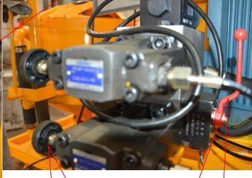
Speed control valve, Adjust the grouting displacement, Clockwise reduce and counterclockwise increase Oil adding part
