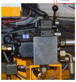
1. Grouting pump speed regulating valve:
