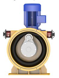
When the rotor unit drives single roller to rotate, hose is squeezed and deformed. After the roller rotate, the deformed hose recover by its elasticity. Thus the negative pressure in this hose is generated, sucking slurries, and discharging through output under rollers' push, finally forms pressure conveying of slurries.
