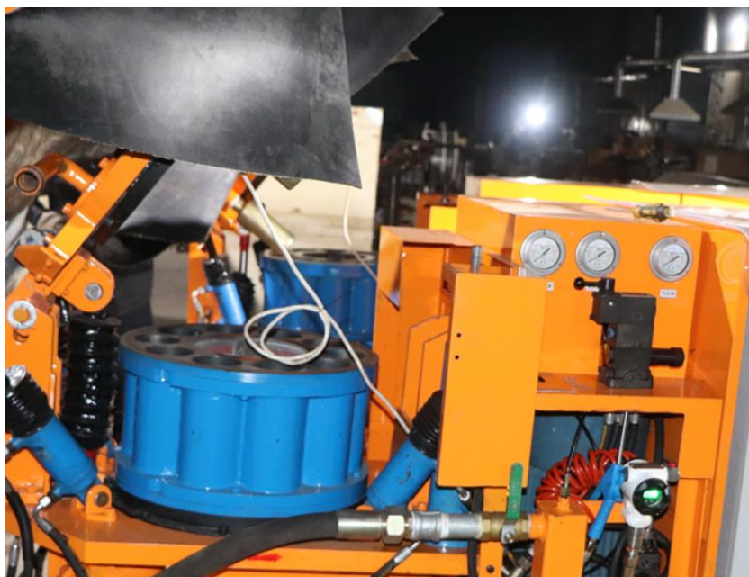
Hydraulic lift the rotor
